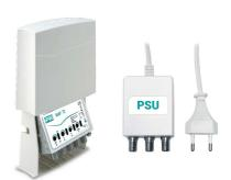
1-input (UHF) mast amplifier with 30dB gain and up to  $118dB\mu V$  output level on UHF band, gain adjustment 0-15dB and low noise figure. 694MHz 5G and 4G LTE integrated filter. Power supply included in the package.
